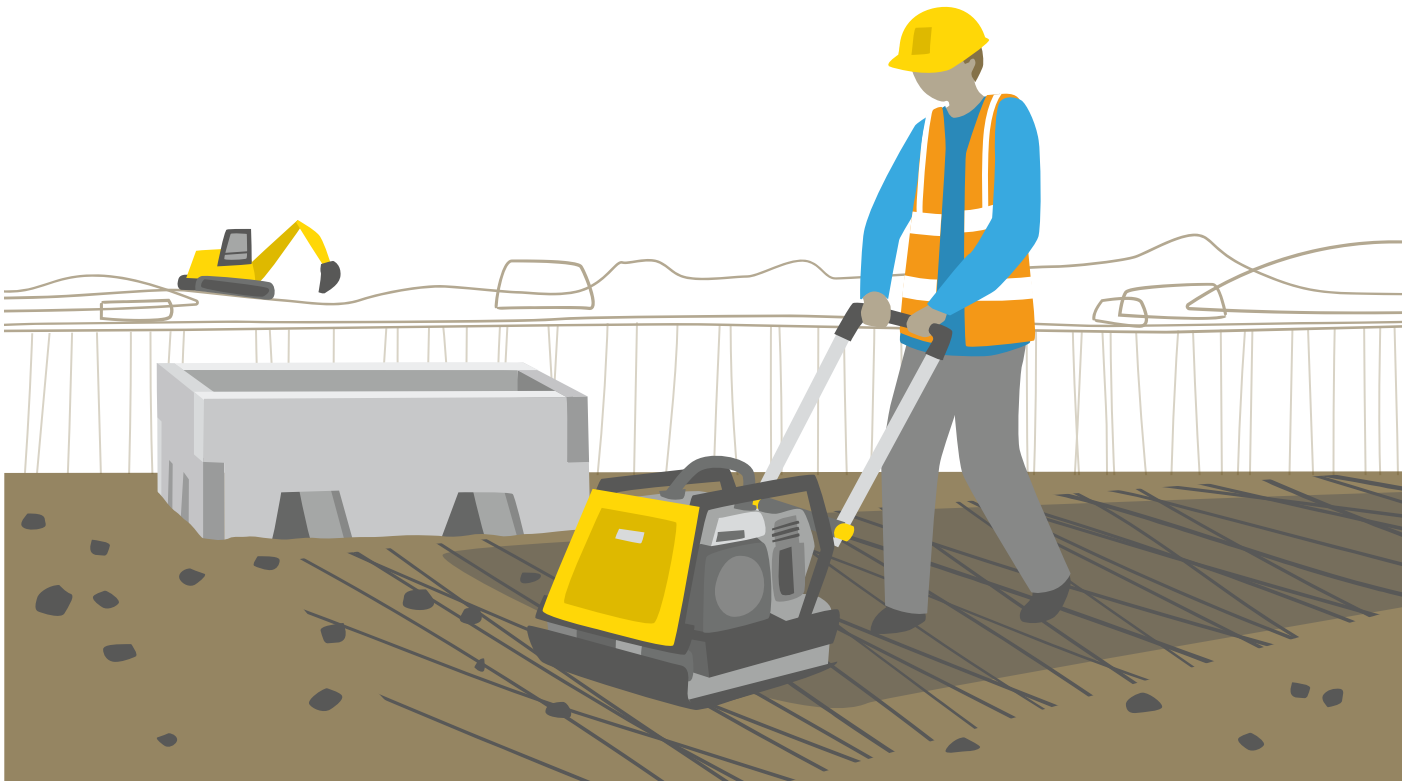
Figure 14: The structural soil is compacted in layers during installation.
